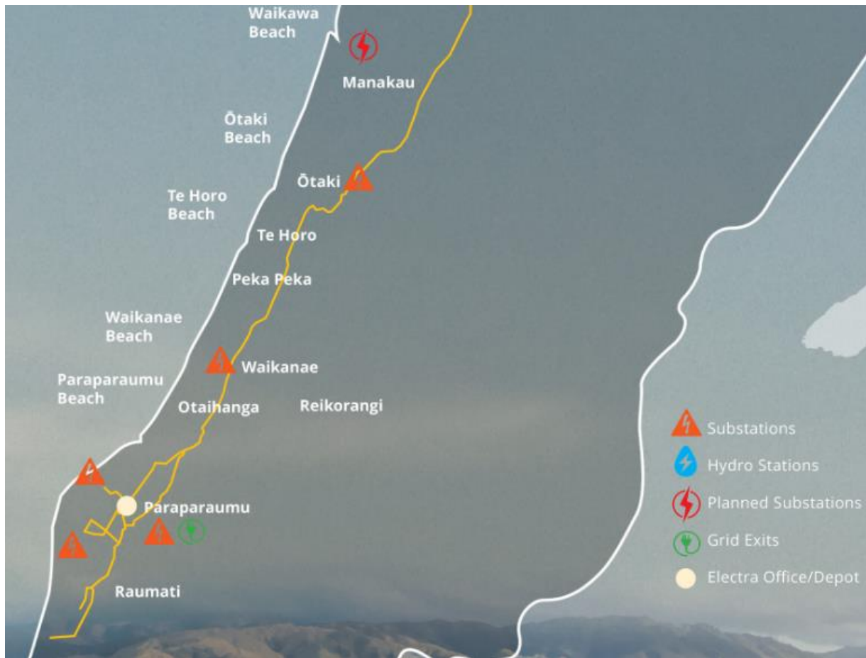
Figure 8. Electra zone substations and interconnecting sub-transmission circuits 12
