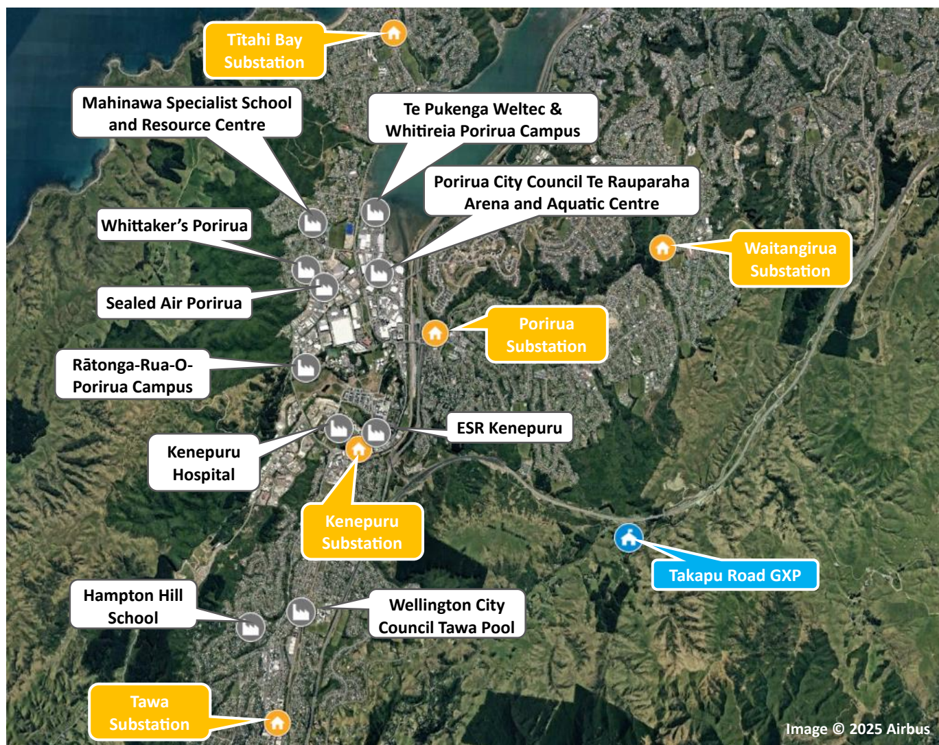
Figure 80. Takapu Road 33 kV GXP: EECA Load Sites vs local substations (northern snippet)
