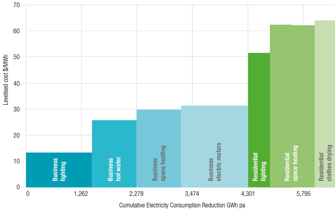
Figure 5: Equivalent LRMC of energy efficient technologies
