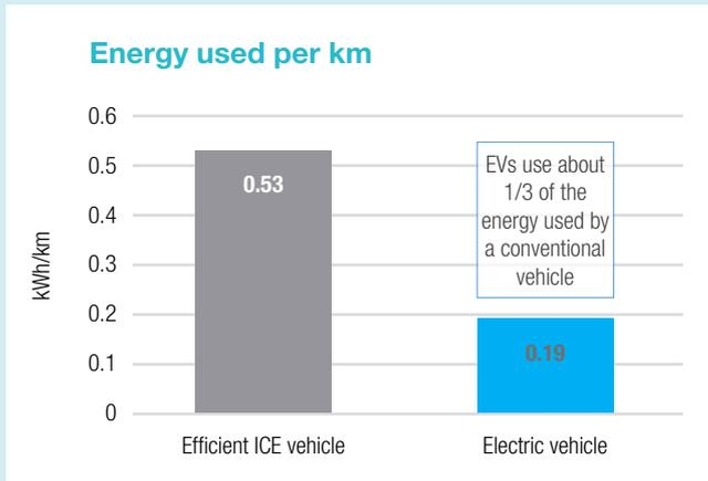
Figure 3: Energy used per kilometre of ICEs and EVs
