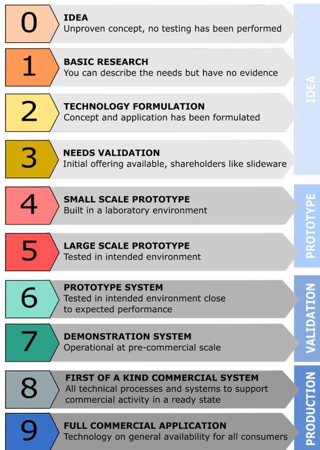
Figure 1.3 Technology readiness level (Drescher et al. 2016).
