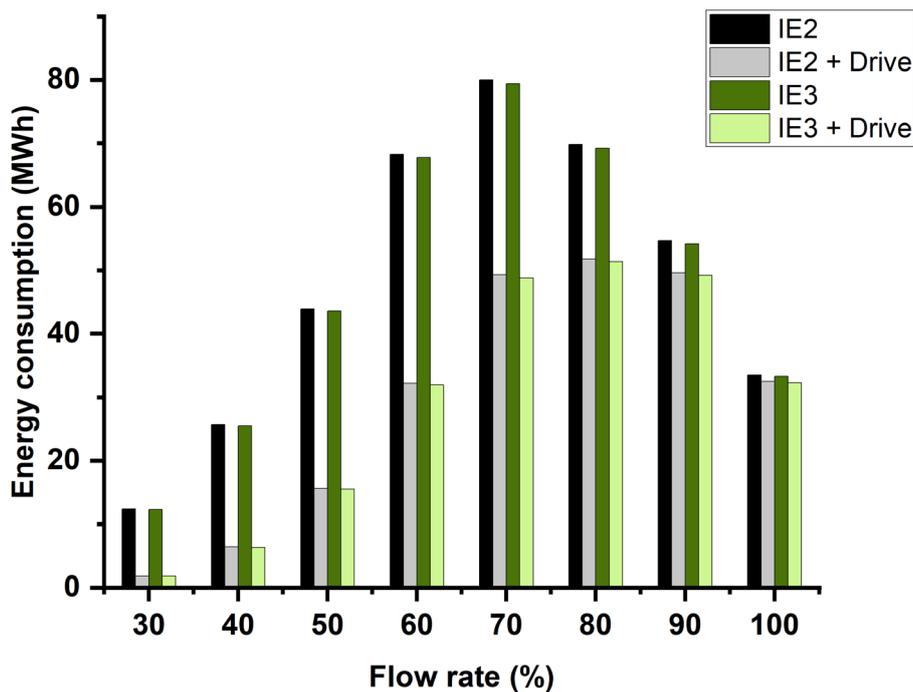
Figure 3.6 Energy consumption for a fan using 170 kW motor with and without a power drive system.
