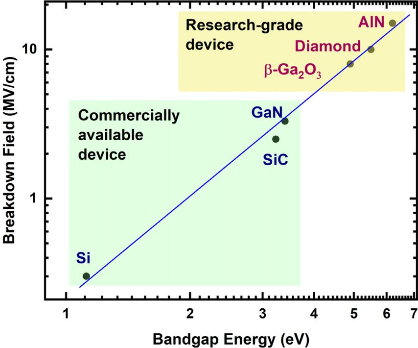
Figure 2.33 Band-gap energy and breakdown field of semi-conductors (Cadeo Group 2020; Zhang et al. 2022; Mariani 2023; Kapp et al. 2024).
