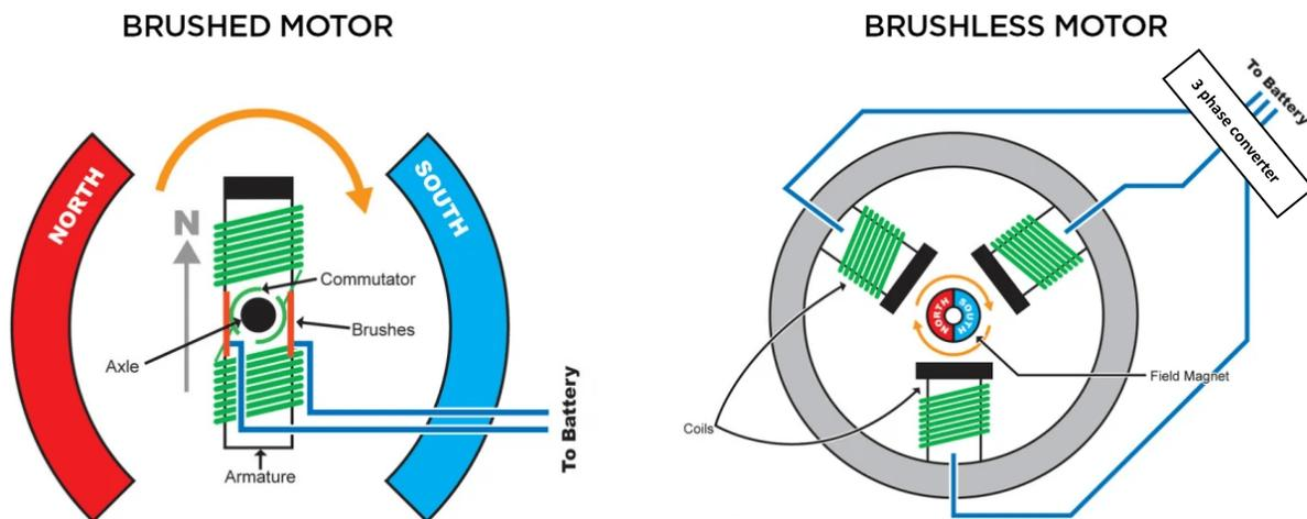
Figure 2.7 Brushed and brushless DC motor types of electric motors (Winstanley 2020).
