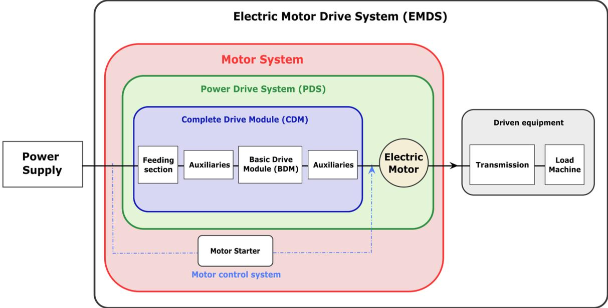
Figure 2.2 Electric motor drive system (IEC 2017, 2014).
