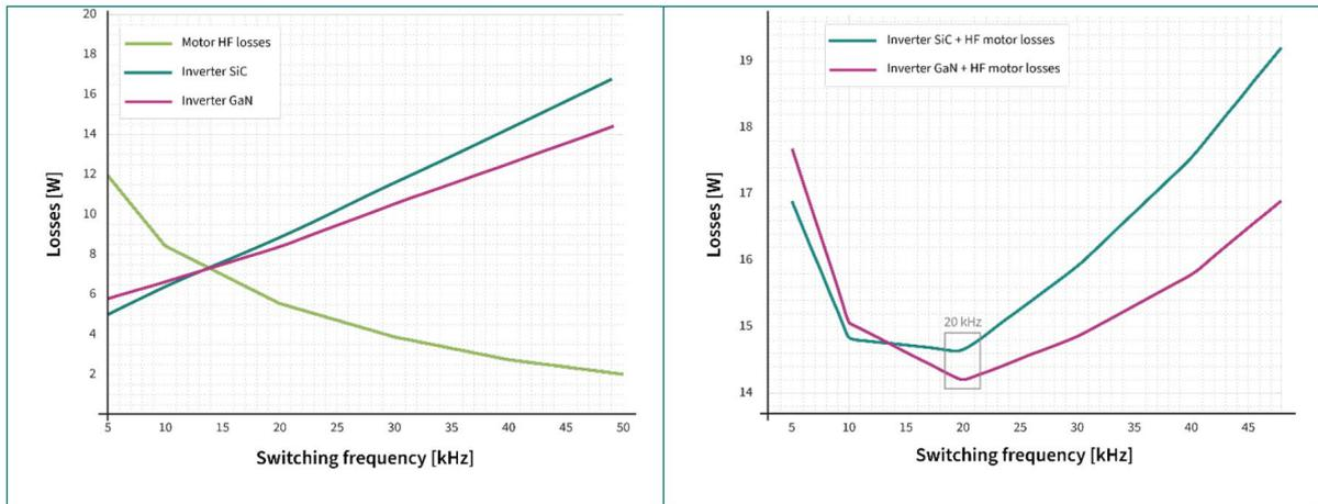
Figure 2.35 Example for motor efficiency with switching speed (Mariani 2023).
