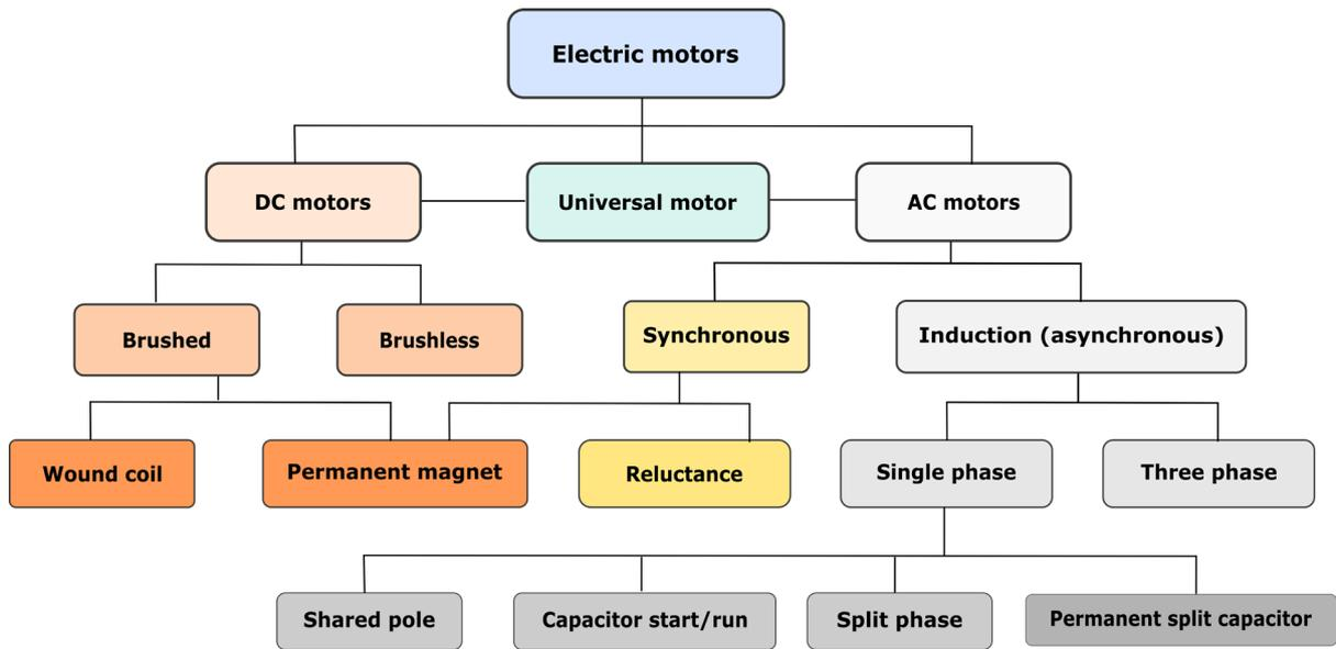
Figure 2.6 Types of electric motors.
