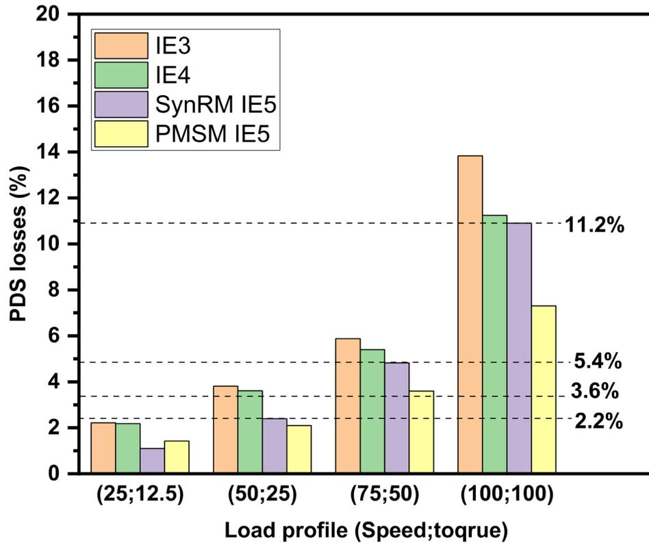
Figure 2.26 Comparison of power drive system losses in electric motors (Fong et al. 2020).
