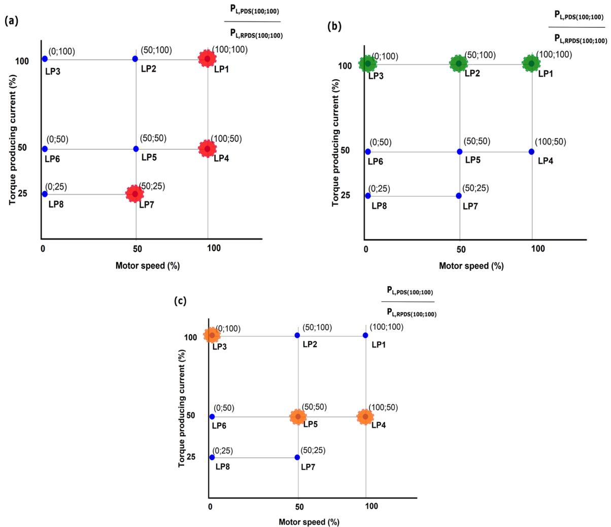
Figure 2.24 Load points for loss estimation for (a) variable load (red circles), (b) constant torque (green circles) and (c) constant power (orange circles) motor applications.
