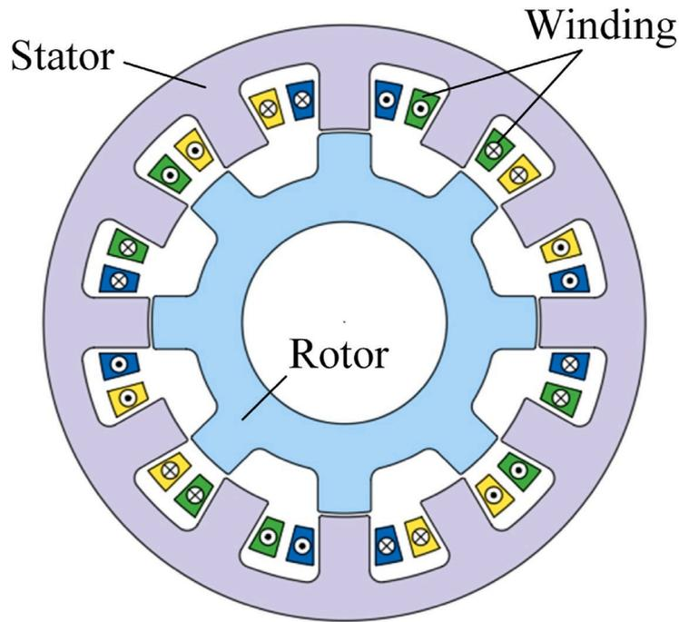
Figure 2.12 A schematic of switched reluctance motor (SRM) topology of a conventional 12/8 SRM (from Feng et al. [2024]).
