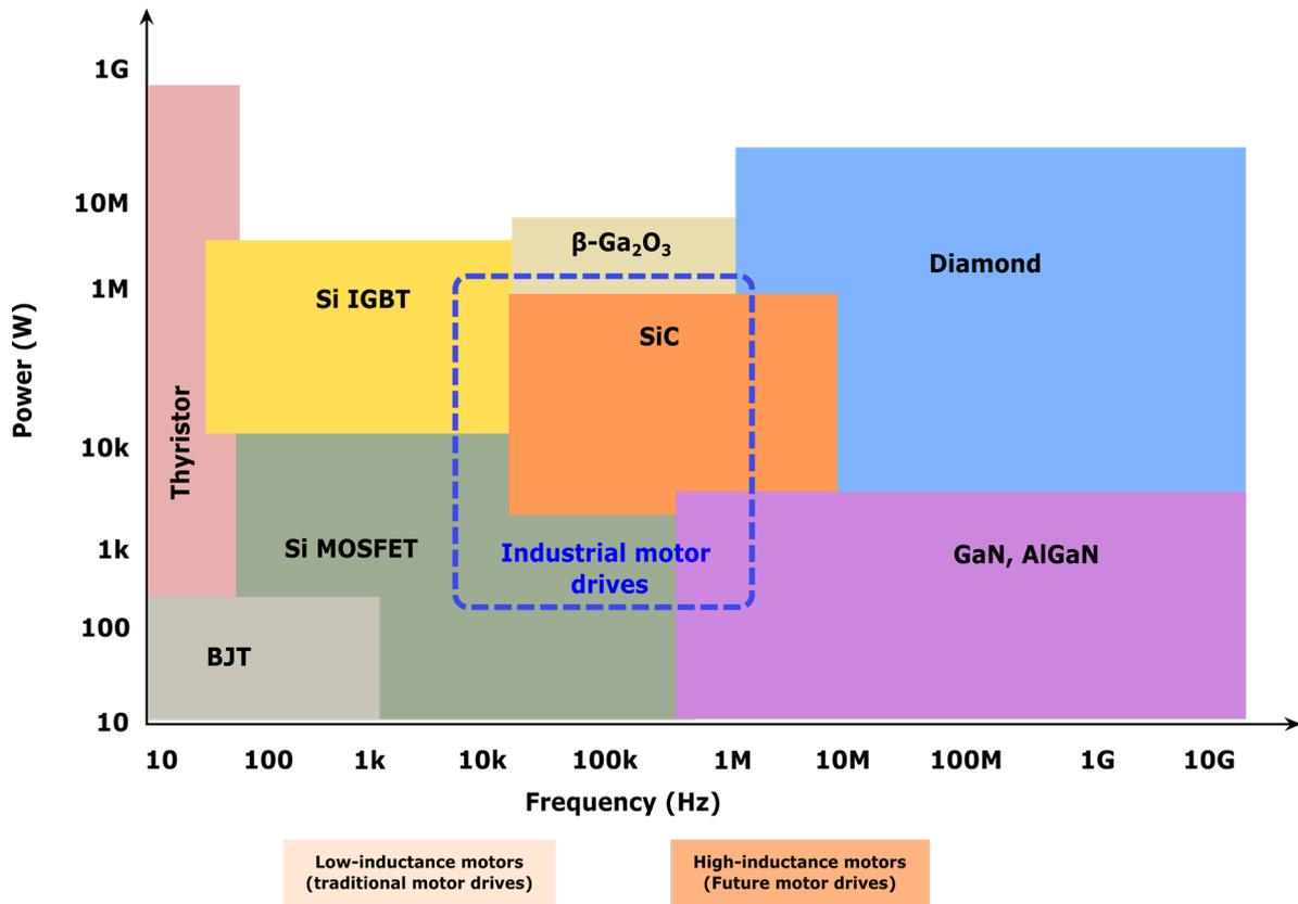
Figure 2.29 Motor drives' switching technologies positioning (Zhang et al. 2022).
