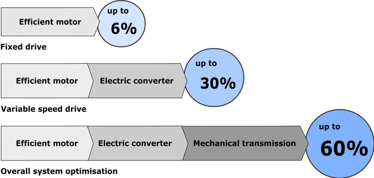
Figure 2.3 Energy saving potential in the electric motor system (Siemens [2024]).
