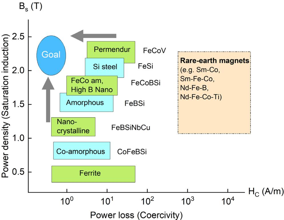
Figure 2.17 Soft magnetic materials (Theisen 2022) and rare-earth-element-based magnets (Trinh et al. 2021) categorised by power density versus power loss.
