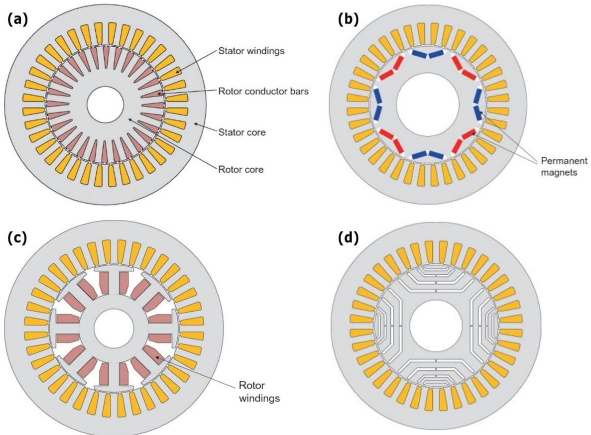
Figure 2.8 Cross-sectional views of different types of motors. (a) Squirrel cage induction motor; (b) interior permanent magnet motor; (c) wound field synchronous motor; (d) SynRM (Shen and Chen 2024).
