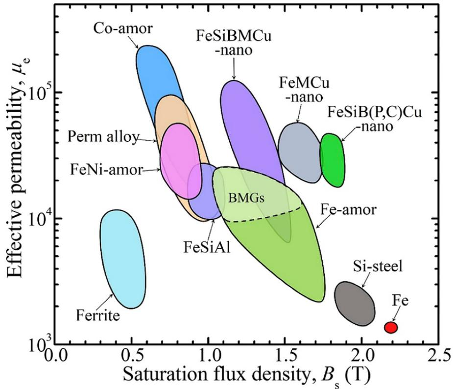
Figure 2.16 Relationship between permeability ( $\mu_e$ ) at 1 kHz and saturation flux density ( $B_s$ ) for soft magnetic materials (Tahanian et al. 2020).
