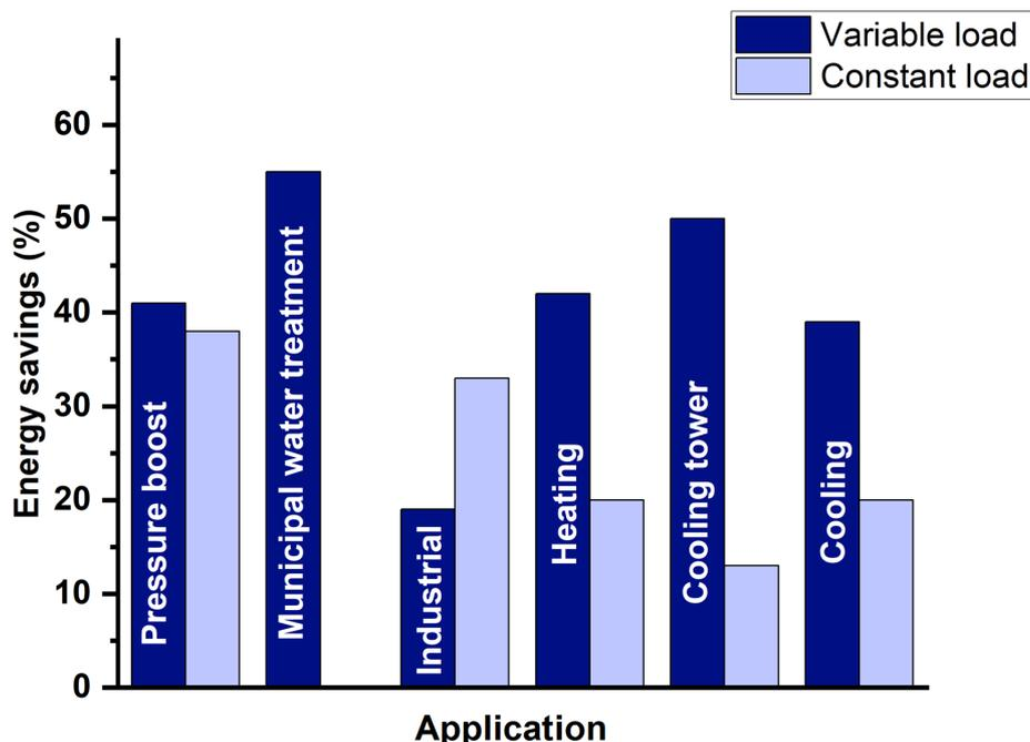
Figure 2.27 Energy savings for various applications at variable and constant load (adapted from Cadeo Group [2020]).
