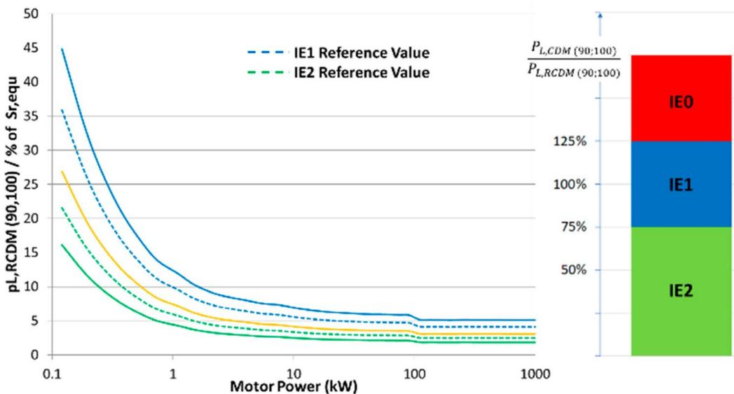
Figure 2.23 Efficiency levels and IE-classes for complete drive modules (IEC 2017, 2024; Fong et al. 2020).
