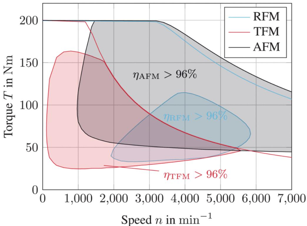
Figure 2.13 Comparison of efficiency in dependence of operation point of permanent magnet synchronous motors as radial flux motors (RFM), axial flux motors (AFM) and transverse flux motors (TFM) (Kaiser and Parspour 2022).
