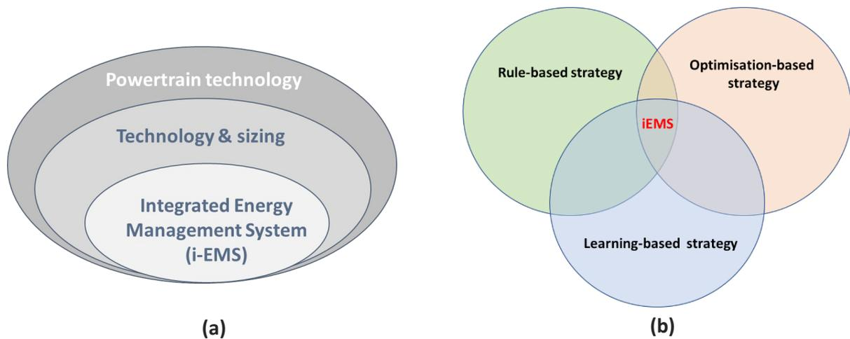
Figure 2.38 (a) System-level design and (b) classification of energy management strategies (Tran et al. 2020).
