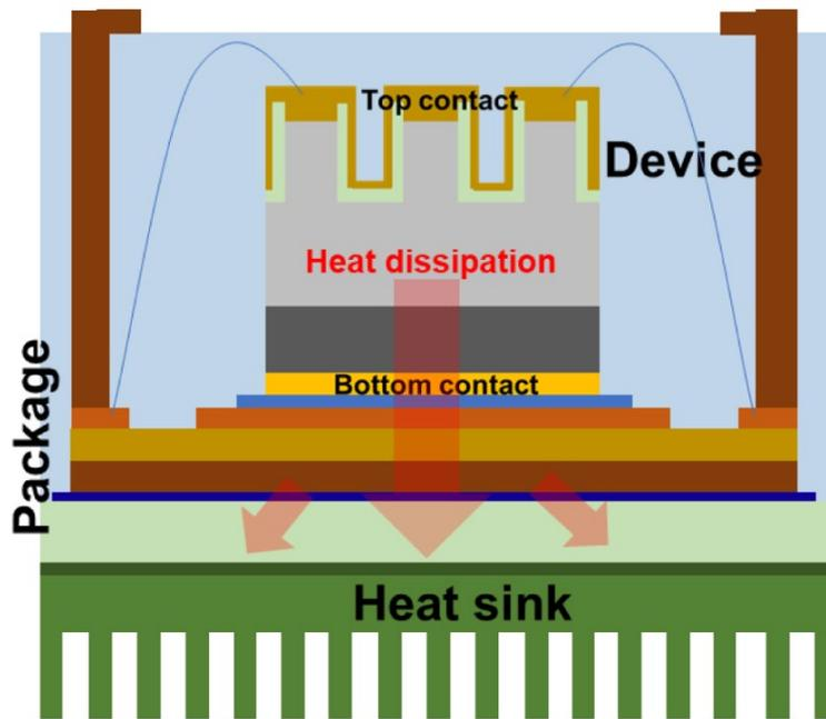
Figure 2.36 Schematic of thermal management and packaging of wide band-gap and ultra-wide band-gap devices (Qin et al. 2023).
