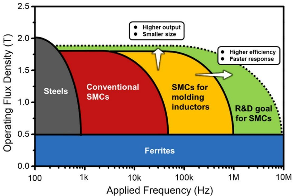
Figure 2.19 Comparison of magnetic materials and the research direction for soft magnetic materials used in alternating current magnetic fields (He et al. 2023).
