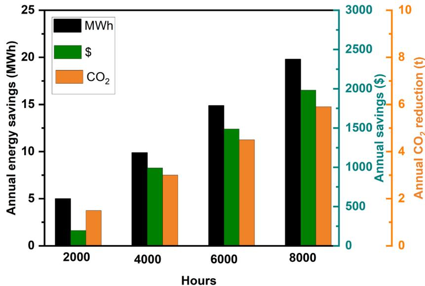
Figure 3.7 Energy and cost savings, as well as CO<sub>2</sub> reduction, for a fan using an 11 kW motor with a power drive system.
