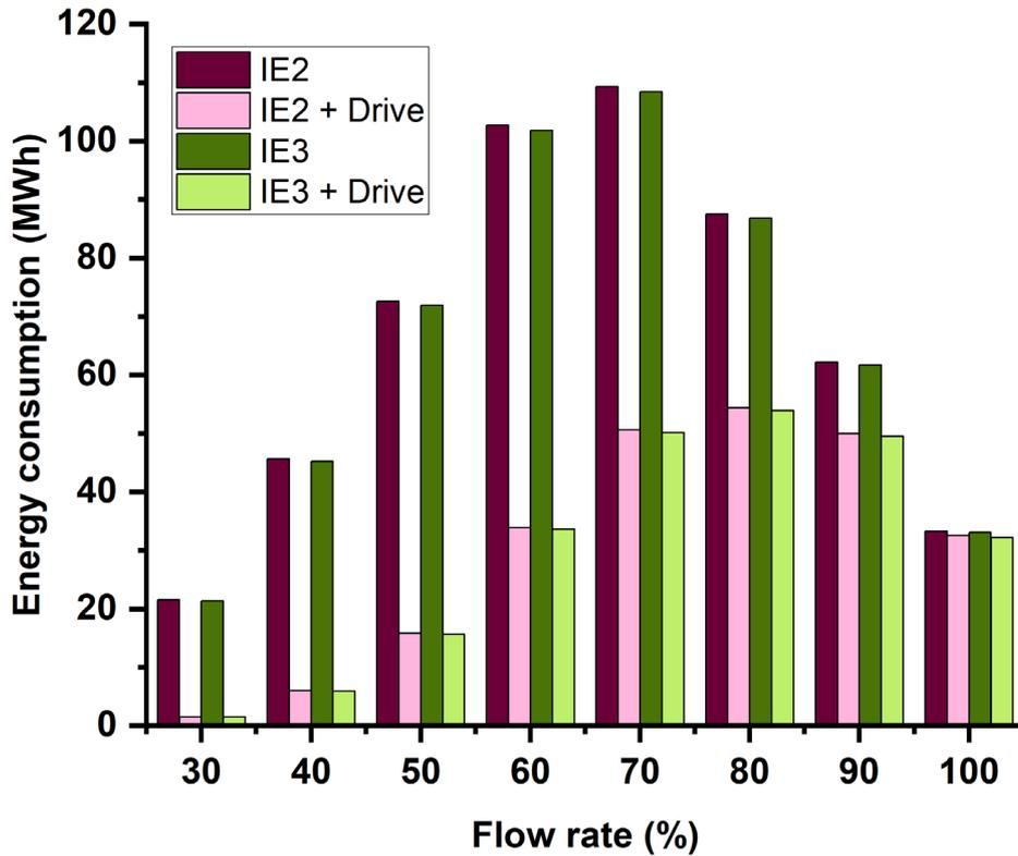
Figure 3.9 Energy consumption for a pump using 170 kW motor with and without a power drive system.
