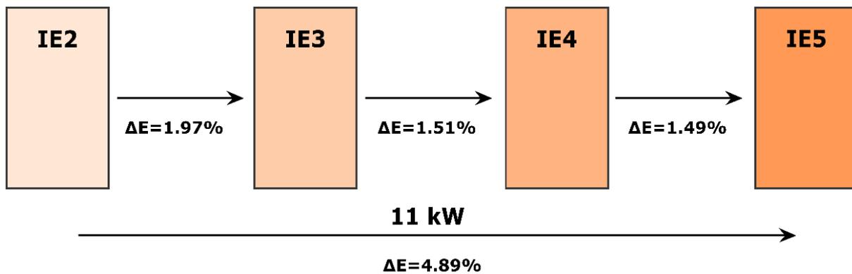
Figure 3.3 Energy savings using IE2, IE3, IE4 and IE5 class 11 kW motors.
