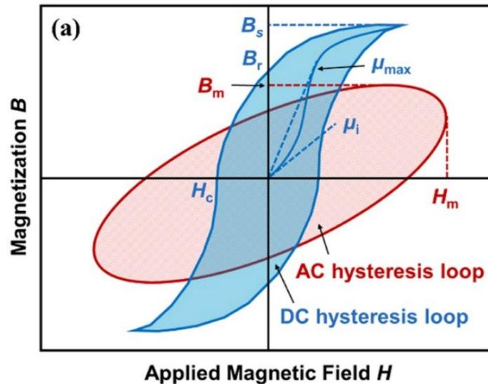
Figure 2.15 Schematic of hysteresis loops of soft magnetic materials obtained by direct and alternating current conditions (He et al. 2023).
