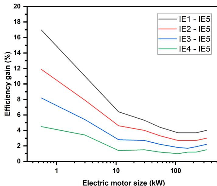
Figure 2.10 Efficiency gain against mid-point power size using IE5 efficiency motors (IEC 2017, 2024).
