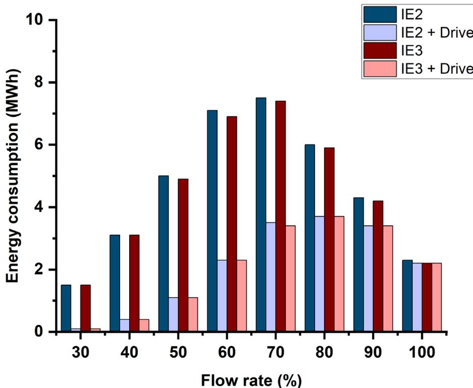
Figure 3.8 Energy consumption for a pump using 11 kW motor with and without a power drive system.
