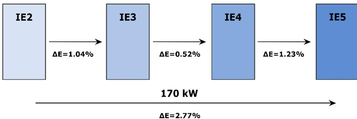
Figure 3.4 Energy savings using IE2, IE3, IE4 and IE5 class 170 kW motors.
