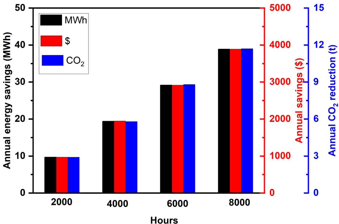
Figure 3.10 Energy and cost savings, as well as CO<sub>2</sub> reduction, for a pump using an 11 kW motor with a power drive system.
