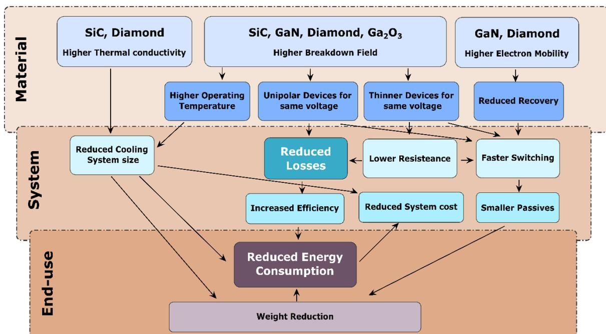
Figure 2.32 Impact of materials' properties on device, system and application performance (Armstrong et al. 2016).
