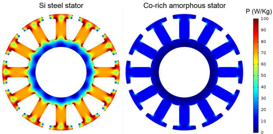
Figure 2.18 Motor stator power loss distribution in stator made of (left) silicon steel and (right) cobalt-rich amorphous alloy (Silveyra et al. 2018).
