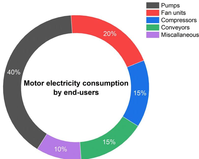
Figure 3.1 Electricity consumption of electric motors by end users (EECA c2024).
