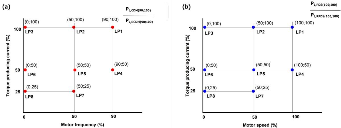
Figure 2.22 Illustration of the operating points for relative loss estimation for (a) complete drive module and (b) power drive system as set in IEC 61800-9 (IEC 2023).
