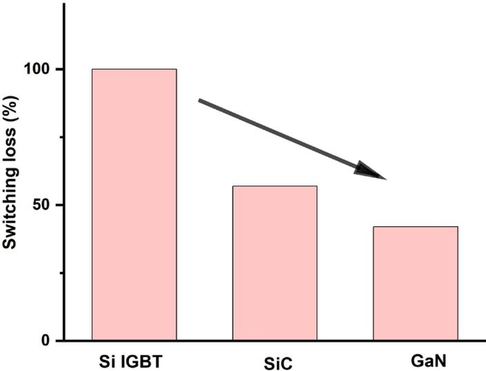
Figure 2.34 Switching loss comparison of Si-IGBT-, SiC- and GaN-based switches (Mariani 2023).
