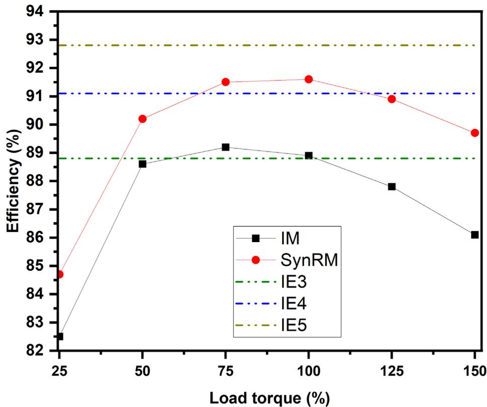
Figure 2.11 Experimental efficiency versus load torque at 400V and 50 Hz (Villani et al. 2022).
