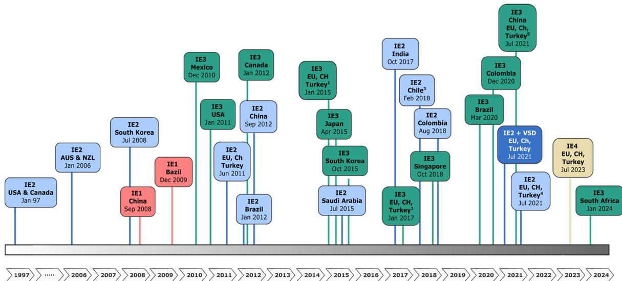
Figure 2.5 Minimum efficiency performance standards adoption for various countries (<sup>1</sup> 7.5–375 kW or IE2 + VSD; <sup>2</sup> 0.75–375 kW or IE2 + VSD; <sup>3</sup> 0.75–7.5 kW; <sup>4</sup> 0.125–0.75 kW; <sup>5</sup> 0.75–1000 kW; <sup>6</sup> 75–200 kW) (De Almeida et al. 2019).
