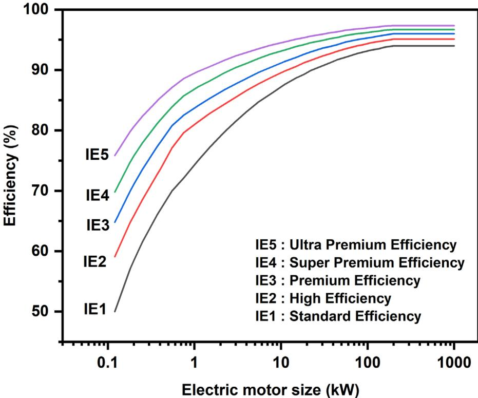
Figure 2.4 Electric motor efficiency for four poles and 50 Hz motors against electric motor size (IEC 2017, 2024).
