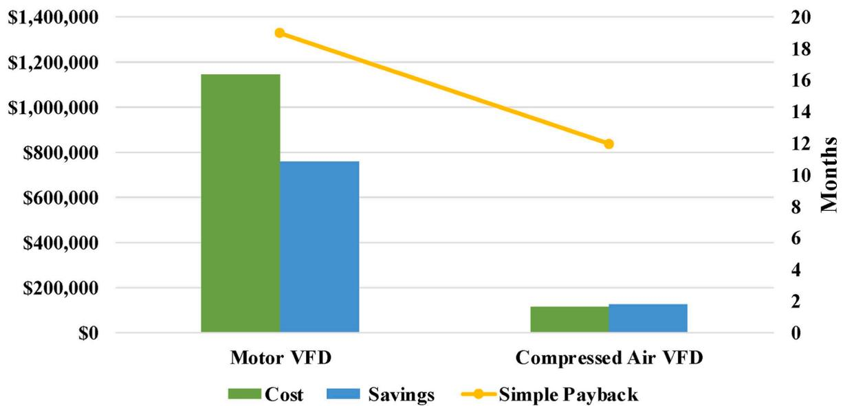
Figure 2.28 Energy savings and payback time for motor and compressed air using VFDs (Kapp et al. 2024).
