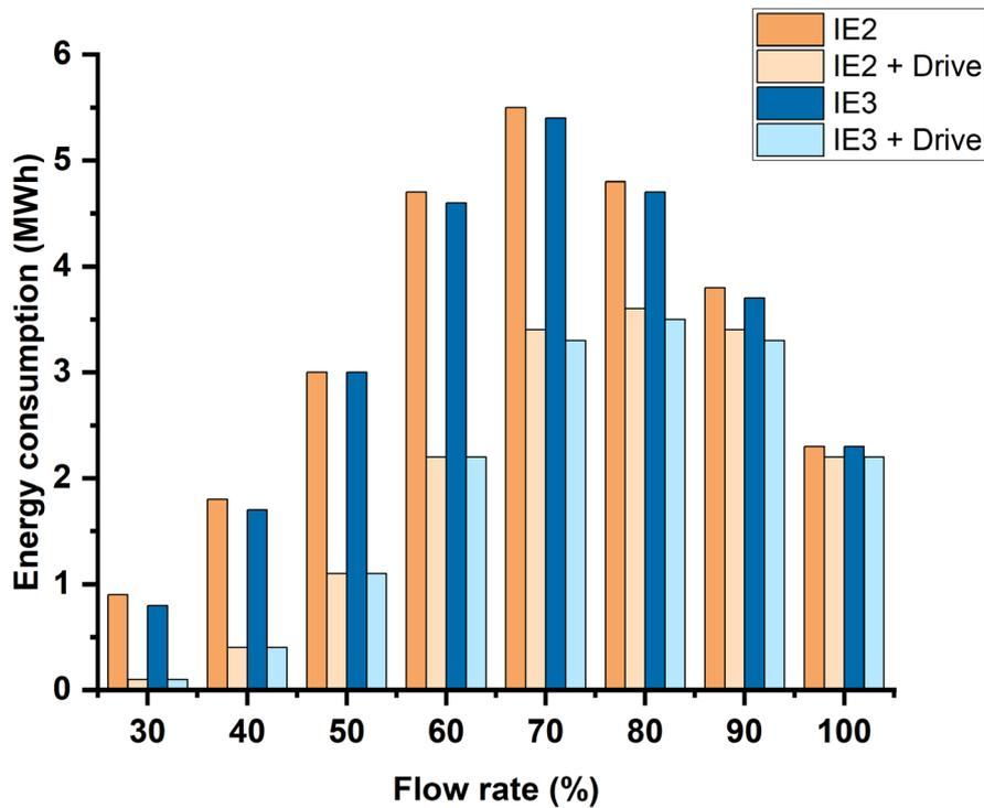
Figure 3.5 Energy consumption for a fan using 11 kW motor with and without a power drive system.
