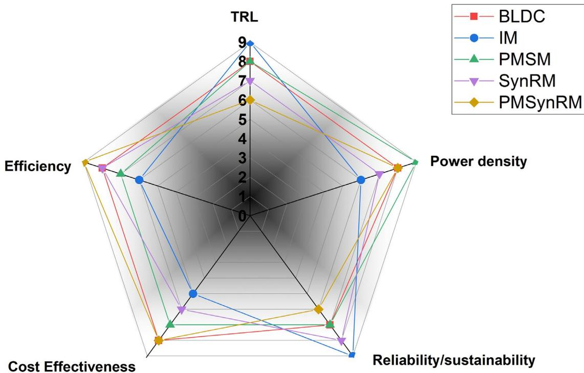
Figure 3.2 Comparison of electric motor performance. BLDC = brushless DC; IM = induction motor; PMSM = permanent magnet synchronous motor; SynRM = synchronous reluctance motor; PMSynRM = permanent magnet synchronous reluctance motor; TRL = technology readiness level.
