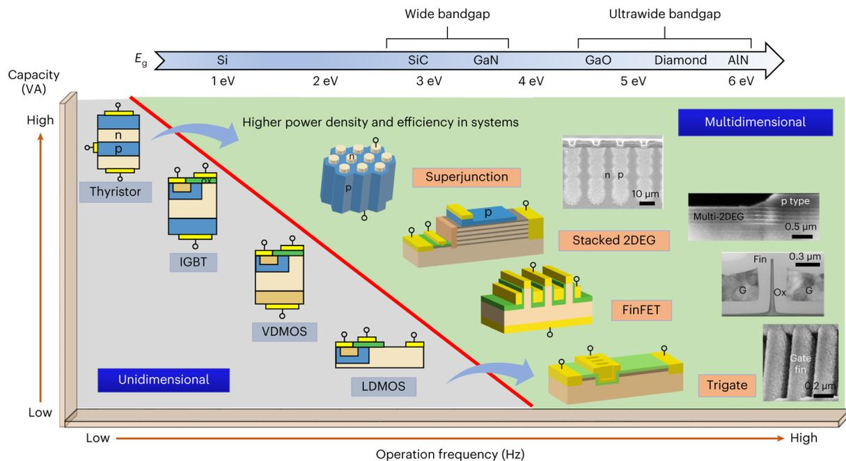
Figure 2.30 Schematic of thyristor, IGBT, vertically diffused MOSFET (VDMOS) and laterally diffused MOSFET (LDMOS) (Zhang et al. 2022). The red line illustrates the approximate limit of 1D power devices (Geng et al. 2023)
