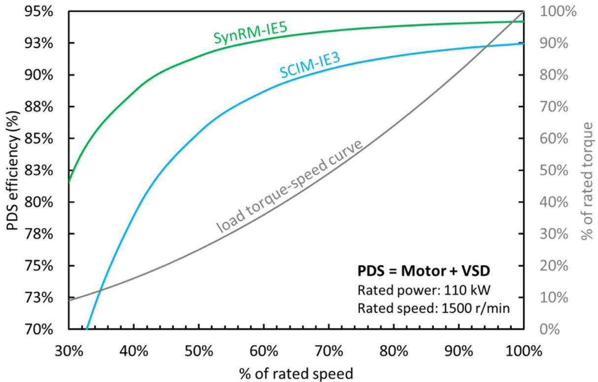
Figure 2.25 Comparison of variable speed drive (VSD)-controlled IE3 and IE5 SynRM motors efficiency (Fong et al. 2020).
