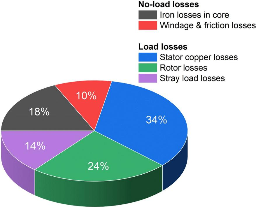
Figure 2.9 Typical fraction of losses in electric motors (Villani et al. 2022; de Almeida et al. 2023).
