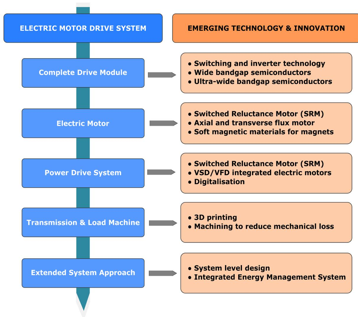
Figure 1.5 Emerging technologies and innovation in electric motor drive systems.
