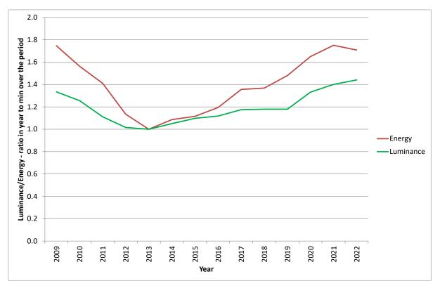
Figure 48: Relative changes in energy and screen luminance for televisions over the period 2009 to 2022 (based on min).
