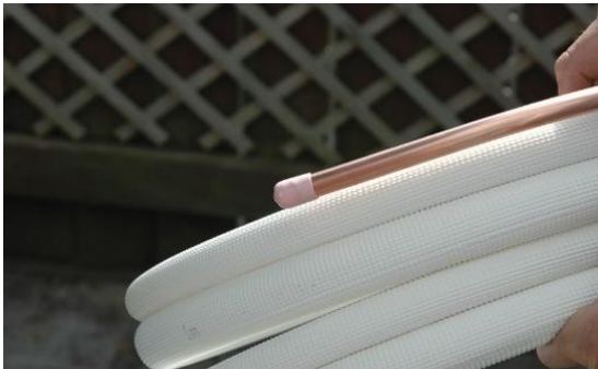
Figure 27: Cover pipe ends
