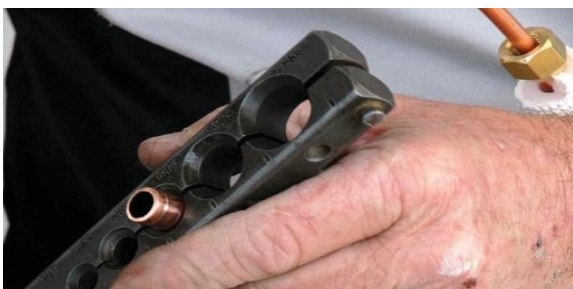
Figure 32: Flare the end of the tube (A)
