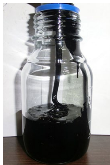
Figure 8: Number 6 bunker oil sample
