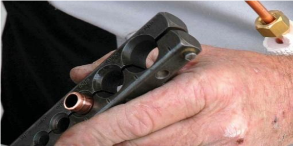
Figure 33: Flare the end of the tube (B)
