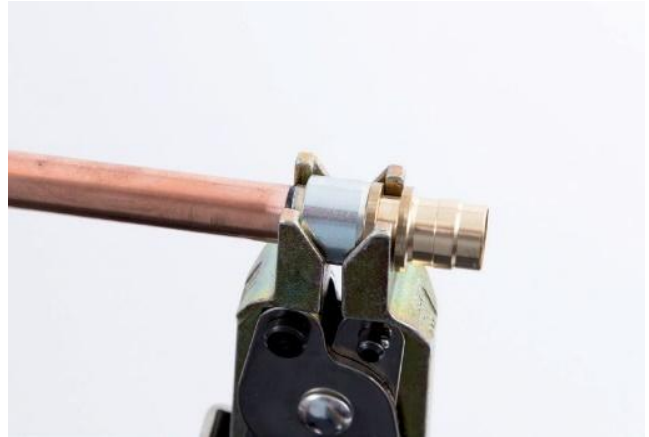
Figure 24: Step 8: Compressing one connection end
