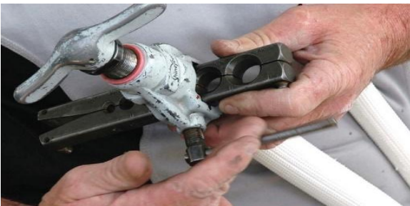
Figure 33: Flare the end of the tube (B)
