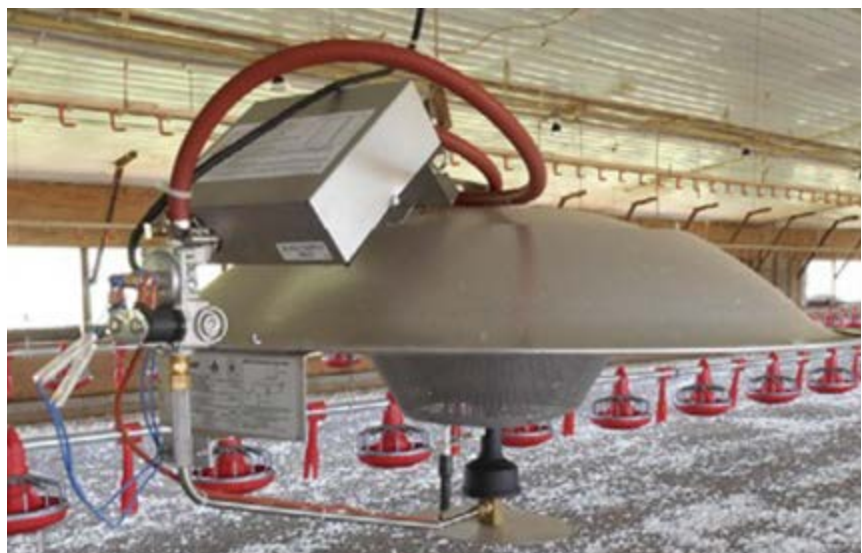
Circular open-flame radiant brooder Image credit: Mississippi State University
