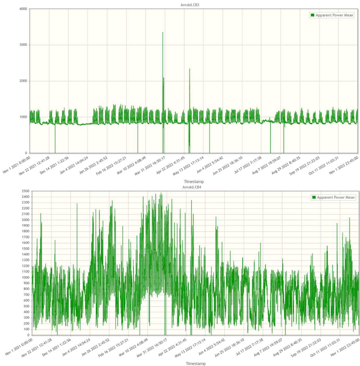
Figure 15 Arnold 33/11kV zone substation: Apparent power (MVA) load characteristics
