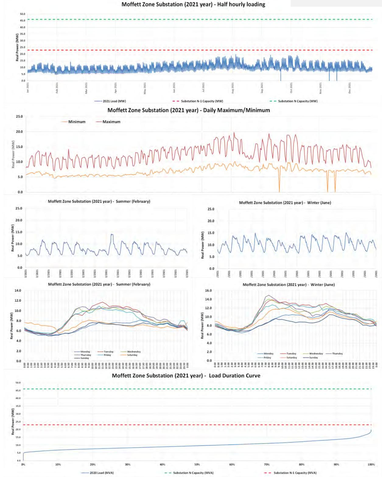
Figure 61 Moffett 33/11kV zone substation: Apparent power (MVA) load characteristics
