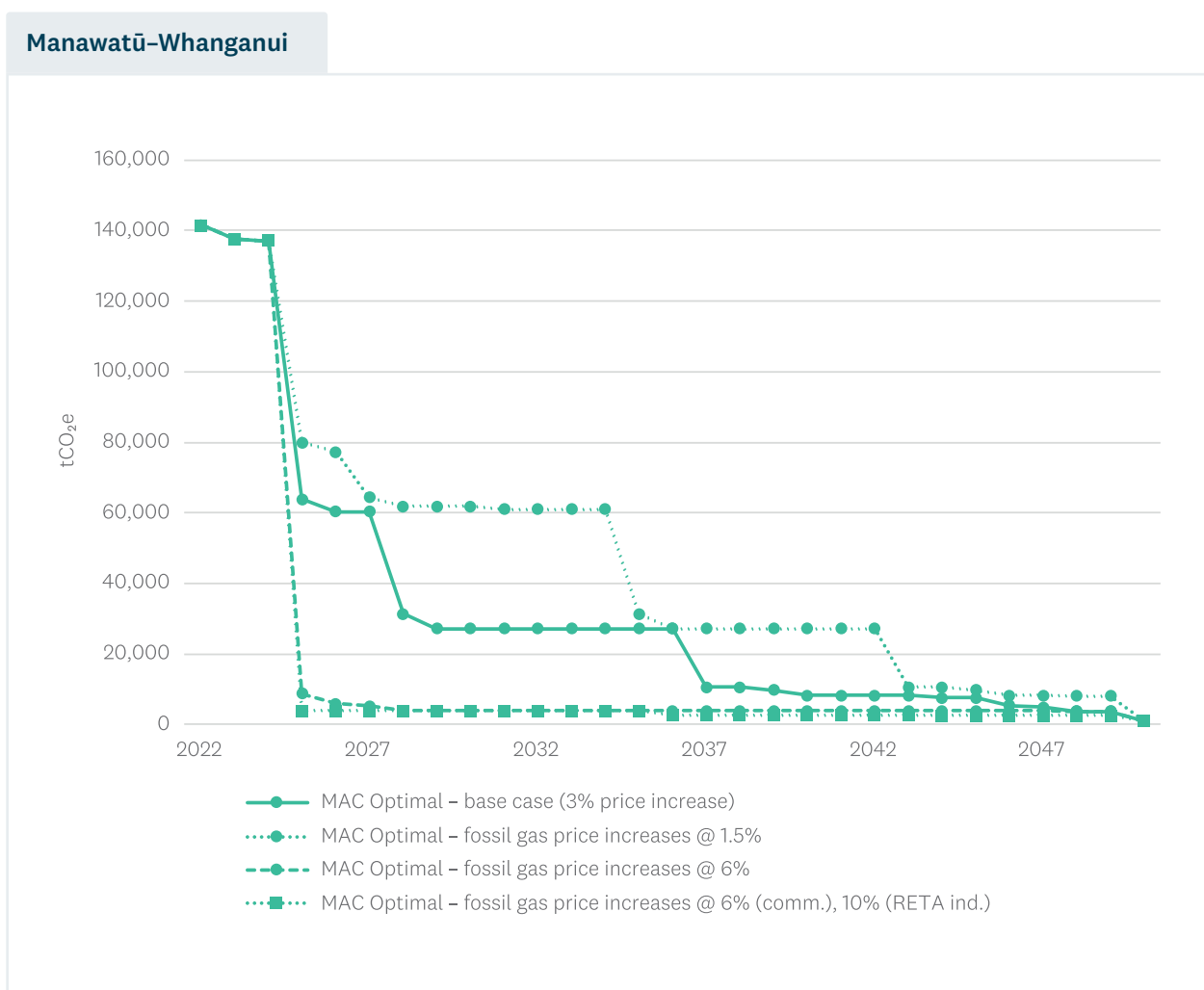
Figure 7 – Sensitivity of emissions reductions pathways to different gas price assumptions.
