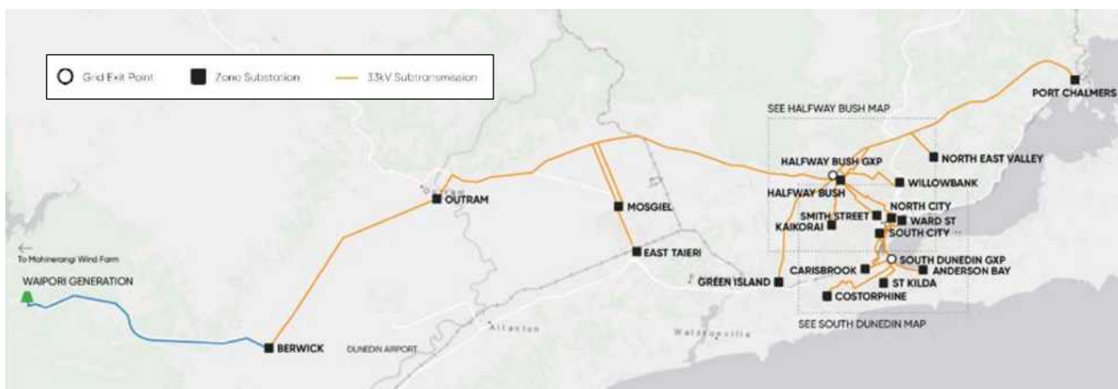
Figure 9 Aurora Energy's Dunedin (Halfway Bush and South Dunedin GXPs) Zone Substation Sub-transmission Diagram 13
