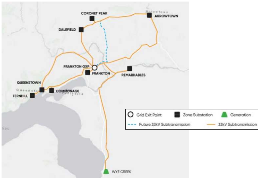
Figure 10 Aurora Energy's Queenstown (Frankton GXP) Zone Substation Sub-transmission Diagram 13
