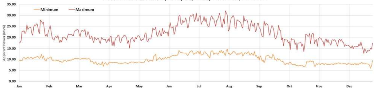
MKAU Zone Substation (2023 year) - Summer (February)
