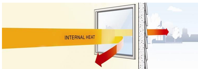
Figure 2: Low-E coating operational demonstration [31]
