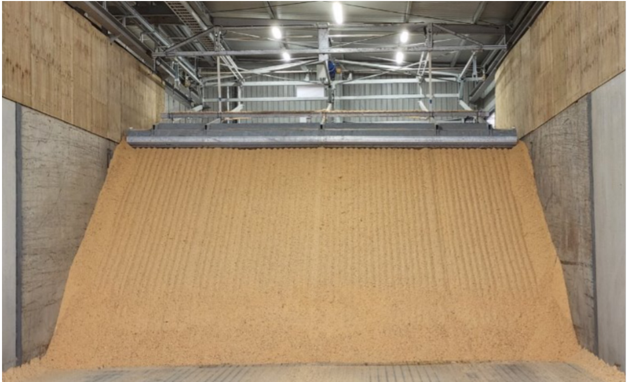
Figure 3: Example of toploader system
