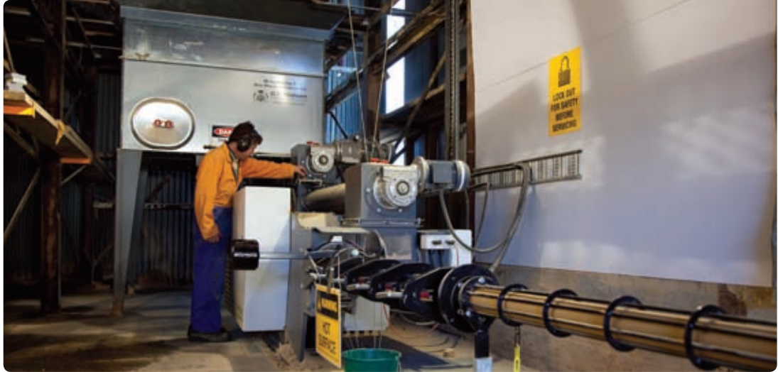
Southern Pine Products' briquette press turns MDF dust into fuel, creating a new revenue stream for the business.
