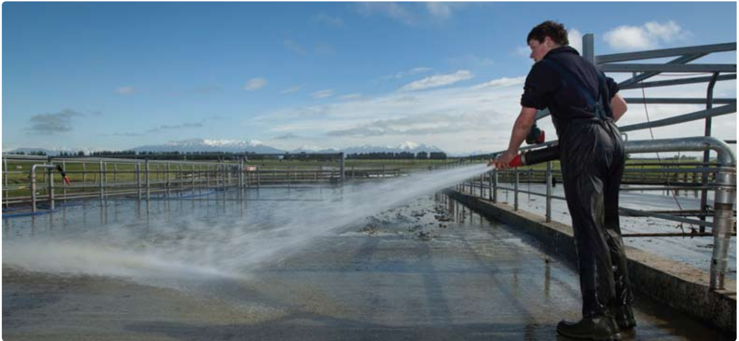
High pressure water cannons minimize wash time and water usage.
