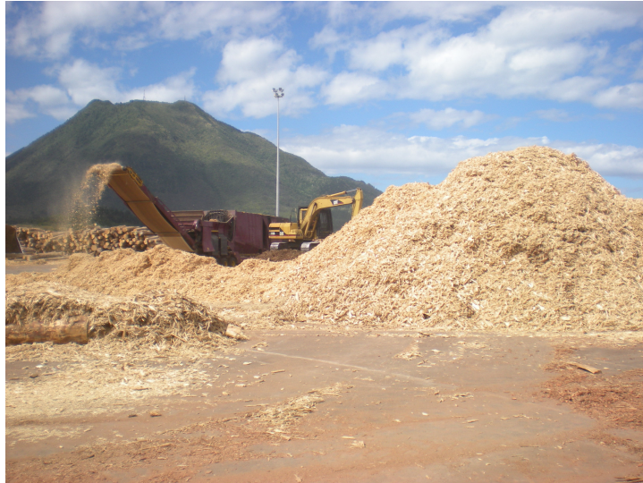
Figure 2: Tub grinder working at the CPY in Kawerau. This CPY processes over 500,000 m 3 of wood annually
