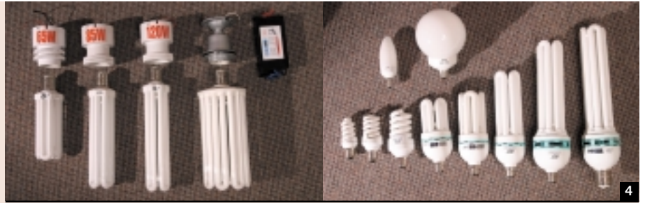
4 XTRA LIGHT'S RANGE OF COMMERCIAL (LEFT) AND DOMESTIC-SCALE (RIGHT) COMPACT FLUORESCENTS. THE LAMPS WITH SEPARATE BALLASTS ARE CHEAPER TO REPLACE, BECAUSE THE BALLAST OUTLIVES THE LAMPS. COSTS IN 2003 RANGE FROM $12 FOR THE SPIRAL 9 W LAMP TO $120 FOR THE 120 W LAMP AND BALLAST.
