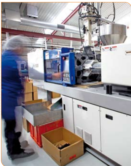
Setting up production on the all-electric injection moulding machines
