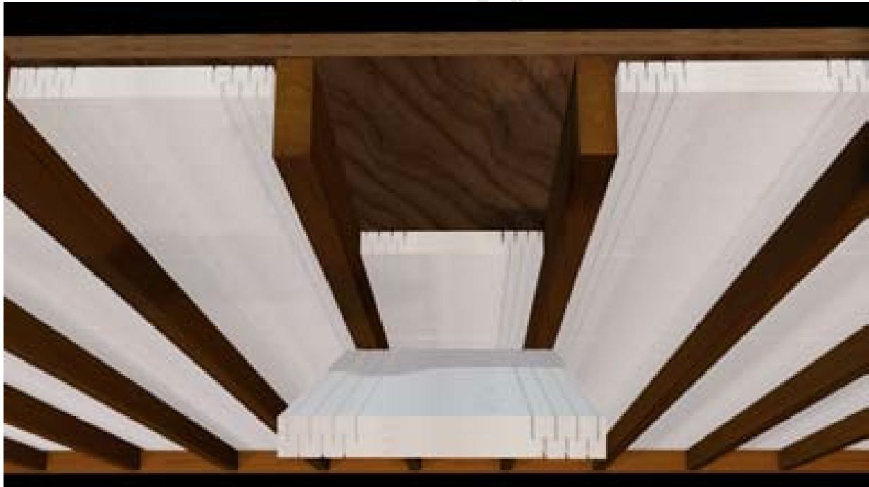
Figure 15 – Installation of underfloor rigid floor insulation
