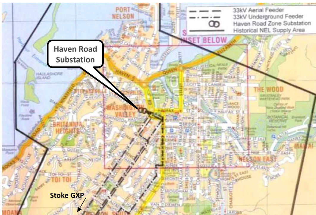
Figure 9 Nelson Electricity: Haven Road 33/11kV substation supplied by four 33kV circuits
